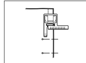
When using a marking pin, always remove it before it can pass under this foot.
