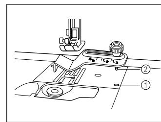
1. Insert the thumbscrew on the seam guide in the screw hole to the right of the needle plate.
