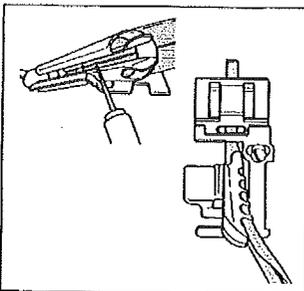
Use a long, narrow object to push the bias tape through the inside of the guide. Pull tape out behind the rear of the foot.
