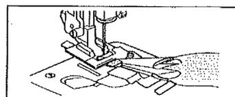
Adjust left-right needle position so that needle is properly lined up with edge of bias tape.
