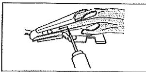
Use a long, narrow object to pull the bias tape through the inside of guide.
