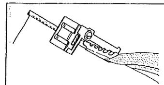
Place the cloth you wish to attach the bias tape to under the needle and align it with the center of the guide. Guide the cloth and bias tape so the tape does not extend over the edge of the fabric.
